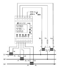
3 wires (2 voltage transformers and 3 current transformers)
