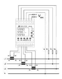
3 wires (2 voltage transformers and 3 current transformers)
