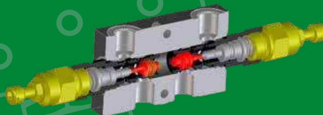
VCB-DL Dual Counterbalance Nose to Nose Design
